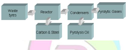
Pyrolysis is a thermo chemical decomposition of organic material at elevated temperatures in the absence of oxygen. Pyrolysis typically occurs under pressure and at operating temperatures about 430 °C (800 °F).
